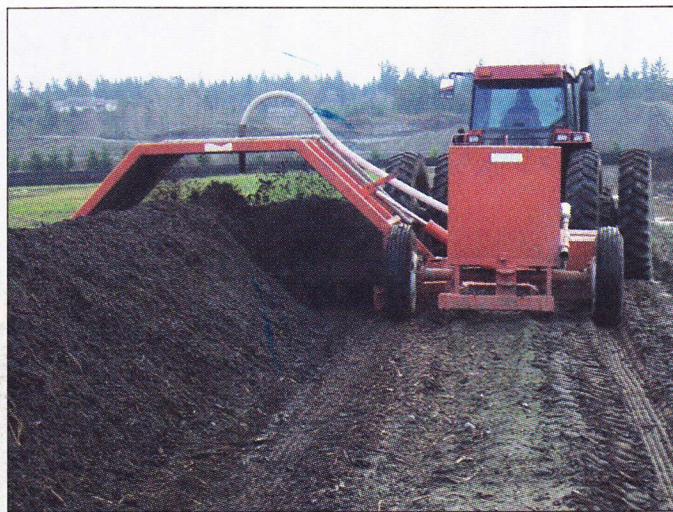
Nash's compost is arranged in long pyramid-shaped windrow piles. A compost turner is used to form the windrows, add water and dairy manure, and aerate the piles.
